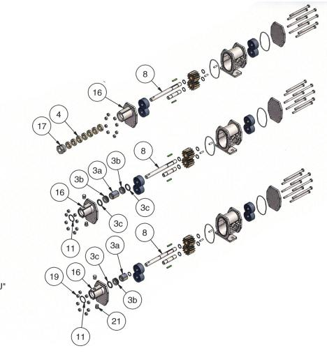
Shaft Seal Codes "N", "P" & "Q" Packing
