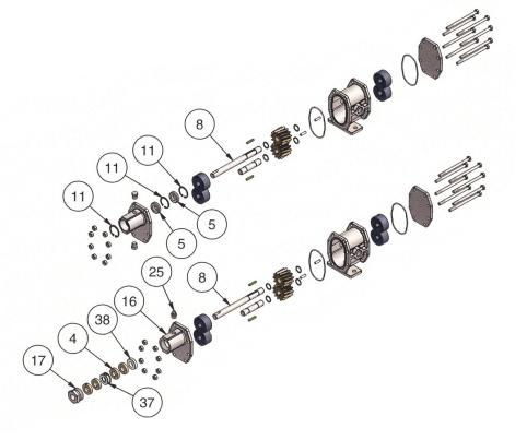
Shaft Seal Codes "R", "S" & "T" Packing with Lantern Ring
