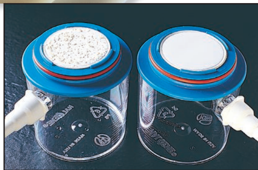
Spallation debris collected onto a microporous filter membrane after recirculating water for 48 hours through TPE tubing (left) and STA-PURE tubing (right).
