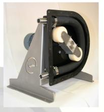
L40 with cover removed, showing its smart roller design which applies a low friction soft compressing action, compared to our competitor's high friction rubbing shoe. The L40's proven roller design also imparts minimal stretch and heat input to the hose, doubling hose life and significantly reducing power consumption.
