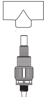
Push the opaque outlet (discharge) tubing onto the compression barb of the Injection/Check valve fitting. Use the tube nut to secure the tube. Hand tighten only.
