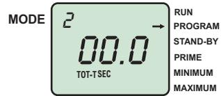
(selected) digit will blink. Note: The left most digit can be programmed from 0 - 19. The decimal is fixed and cannot be moved.
