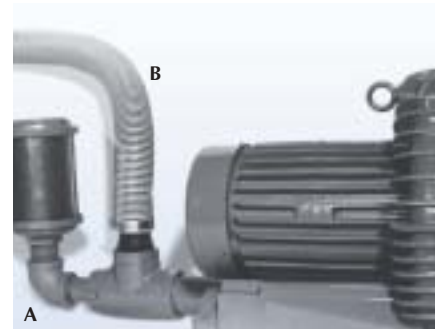
(A) Cooling air flow; (B) Main suction line (may be dead-headed)
